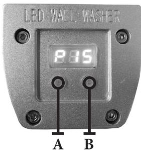
1. This program will allow all lights that are inter-connected with DMX cabling to operate in synchronized unison with the unit assigned as the Master.
