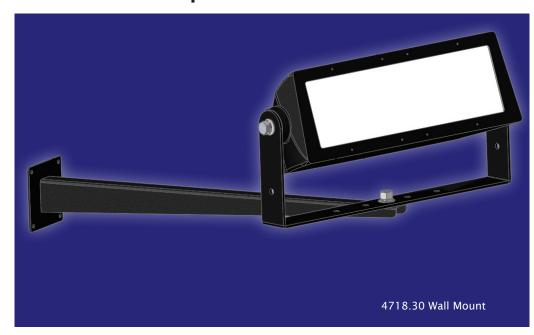
These Wallmounts are made of rugged heavy gauge steel, plated for corrosion resistance and then treated with epoxy powder coat in a black texture to match the Compact Reach Luminaire.
