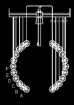
The diagram to the left shows how a crystal chandelier is assembled. Two crystals can be hung on each wire, except in the middle circle of wires (circle F in the diagram)
