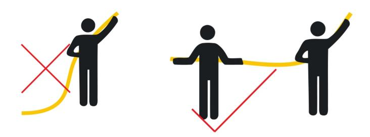
During installation, make sure the light is not twisted, don't knock on the light when put it into the profile.
