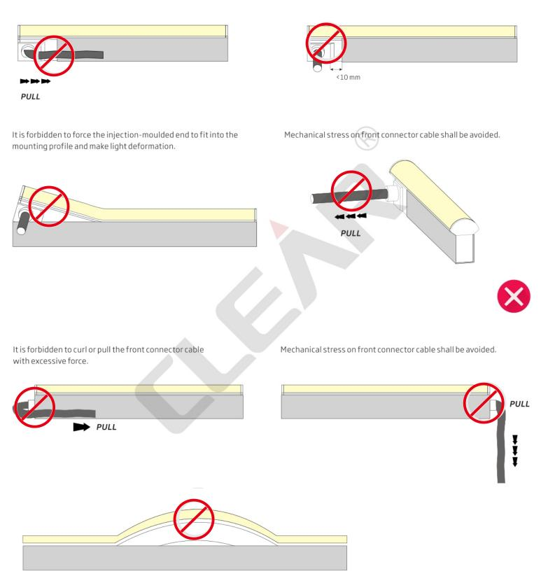
Install the light in one direction, no matter what kind of connector used. Don't let it choke in middle.
