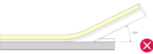
The circuit board could be damaged if installing angle larger than 15 degree.
