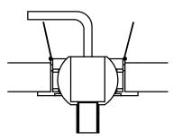
(2)Bend back springs and push into cut out hole.
