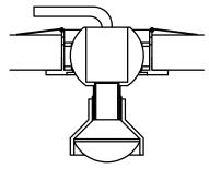
(5)A wide beam of light is produced when the trumpet is screwed on most of the way.
