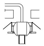
(1)Gently hold fibre optic tail in one hand and screw fitting onto ferrule as far as it will go.
