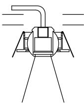
(2)A narrow beam of light is produced if the fiting is screwed on by a few threads.
