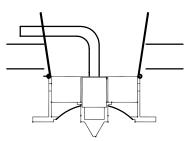
(2)Bend back the springs and push fitting into cut out hole.
